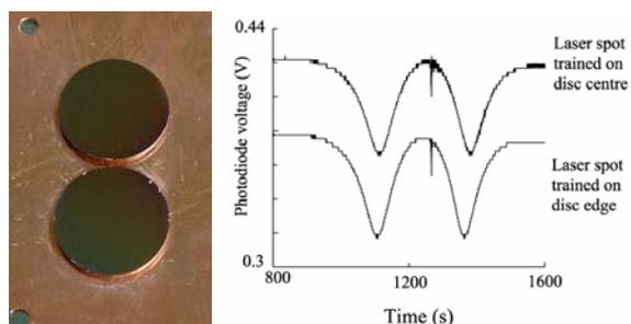
Fig.1- Silicon discs before and after deposition, and interferometry traces taken during deposition.
