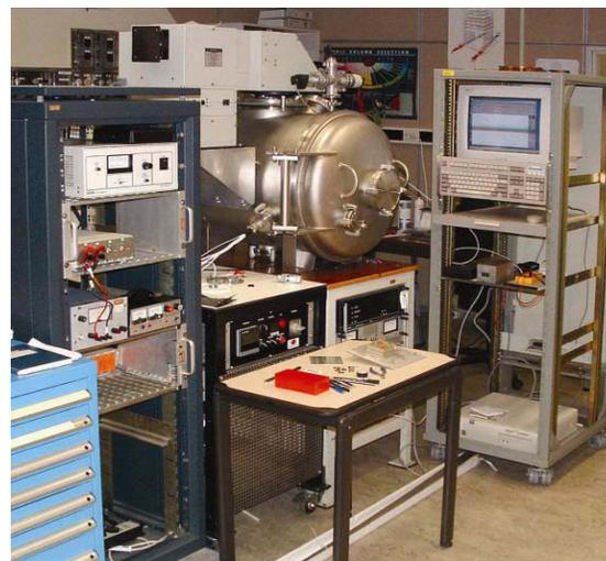
Fig.2- The vacuum chamber and its support equipment. The UV lamps are internal to the chamber [1].
