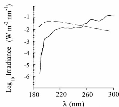
Fig.3- The spectrum of the light used to irradiate the glycine samples (dashed line), compared to a modeled mean martian equatorial surface flux [2] (solid line).
