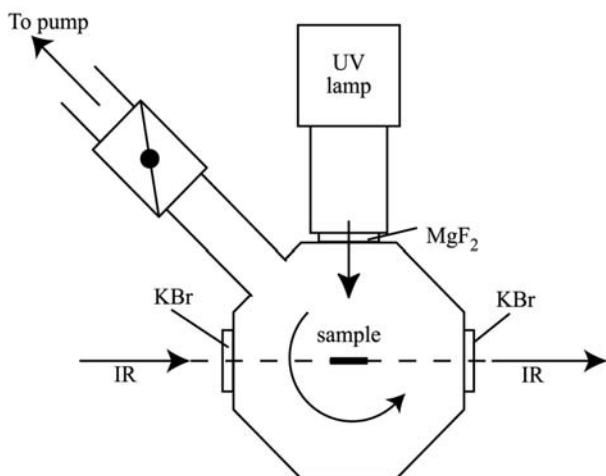
Fig. 3. A schematic drawing of the simulation chamber.
