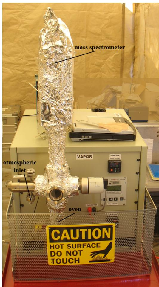
Figure 1. The VAPoR Field Unit.
